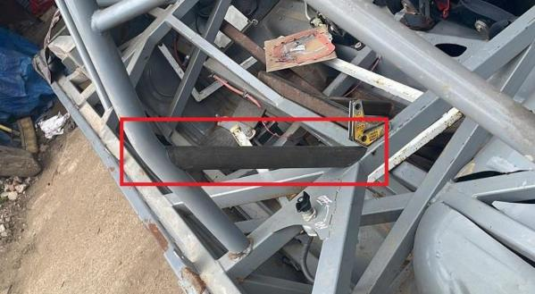
Additional bracing is required to A & B pillar hoops. i.e. to the dash bar and the cross bar behind the
